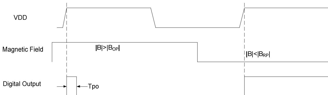
Note:  $V_{DD}$  rise time <1us,  $T_{po}$  is the time from  $V_{DD}$  becoming stable to output becoming valid.
